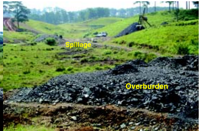
Fig 8 Overburden from mining pit causing spillage to productive lands
